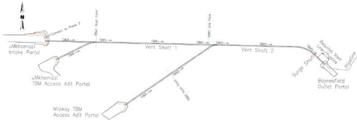
Figure 1. Tunnel alignment and project overview.
