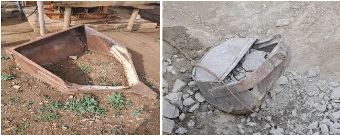
Figure 3: (a) normal scraper scoop (b) modified scraper scoop into a bucket
