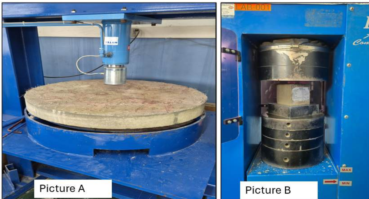
Figure 2: Picture A illustrates the energy absorption round determinate panel sample test, and picture B illustrates the cube samples test for UCS.
