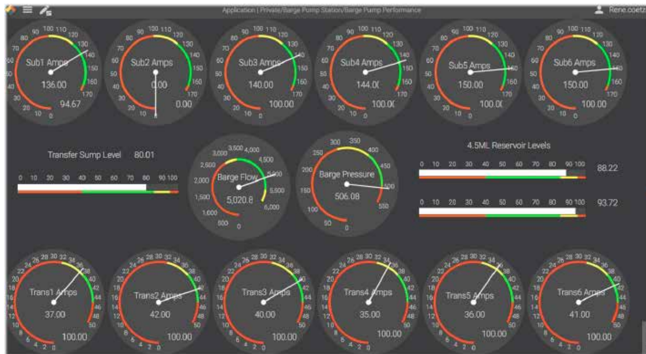
Figure 1: Return water pumping system displaying plant performance in real-time
